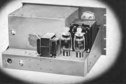
Rear view of the cathode-driven linear amplifier shows the rf enclosure and power supply components.
